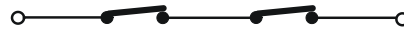
Connection of two N.C. contacts in series (e.g. Photocells, Stop, Edge, etc.)
